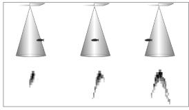
Transducer Cone and Fish Arches
